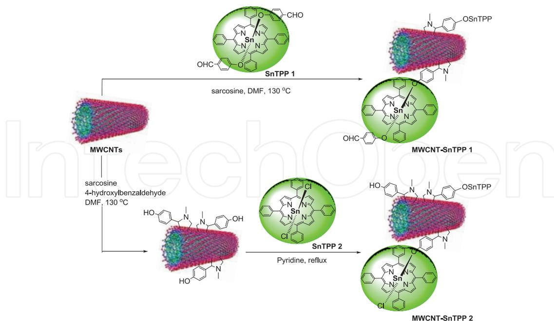
**Scheme 6.** Preparation of MWCNT-SnTPP 1 and MWCNT-SnTPP 2 [44].
