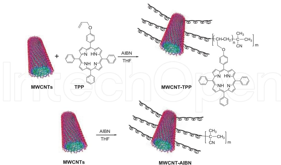
**Scheme 4.** Synthetic routes of MWCNT-TPP and MWCNT-AIBN [42].
