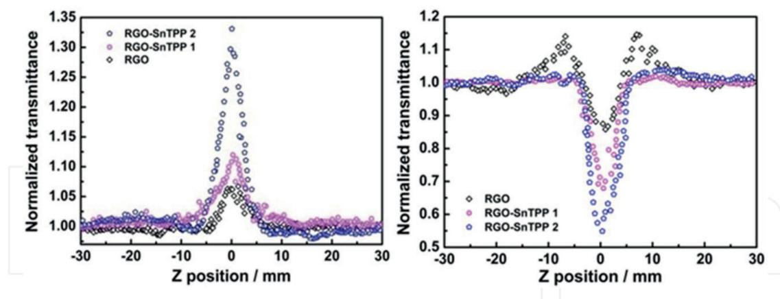
**Figure 8.** Left: Open-aperture Z-scan traces of RGO, RGO-SnTPP 1, and RGO-SnTPP 2 in dimethylsulfoxide (DMSO), obtained under 21 ps, 532 nm laser excitation. Right: Open-aperture Z-scan traces of RGO, RGO-SnTPP 1, and RGO-SnTPP 2 in DMSO, obtained under 4 ns, 532 nm laser excitation [30].
