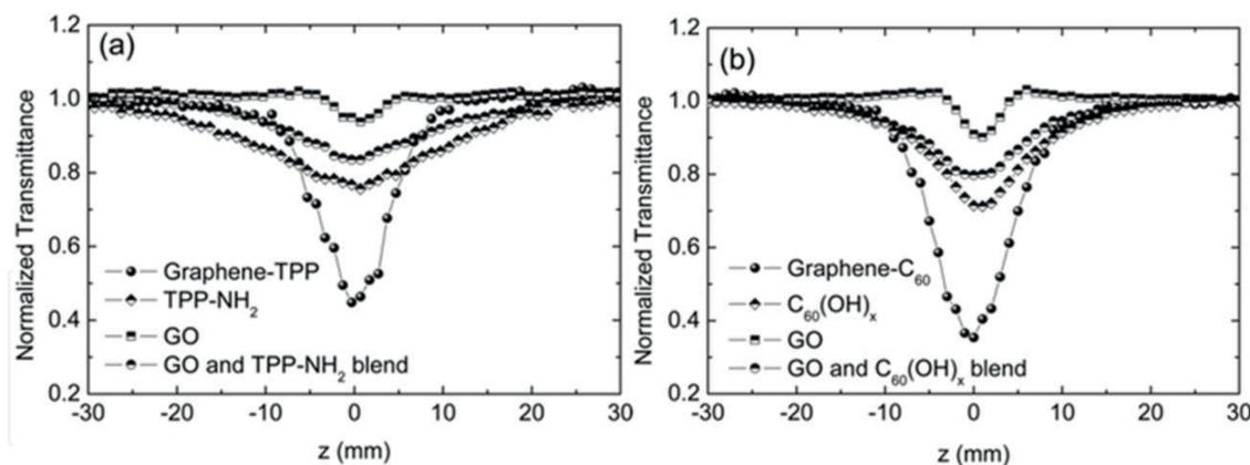
**Figure 5.** Open-aperture Z-scan curves of (a) Graphene-TPP, TPP-NH<sub>2</sub>, GO, and GO and TPP-NH<sub>2</sub> blend, and (b) Graphene-C<sub>60</sub>, C<sub>60</sub>(OH)<sub>x</sub>, GO, and GO and blend C<sub>60</sub>(OH)<sub>x</sub> [25].
