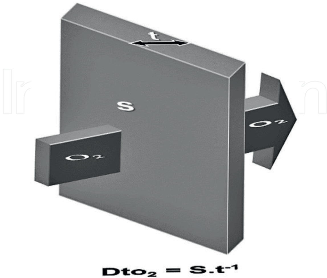
Figure 12. The main parts of a gas exchanger. Oxygen ( O_2 ) diffuses across a tissue barrier under a partial pressure gradient (large arrow). The conductance of the barrier to O_2 ( D_{to_2} ) correlates directly with the surface area ( S ) and inversely with the thickness of the barrier ( t ): equation.
