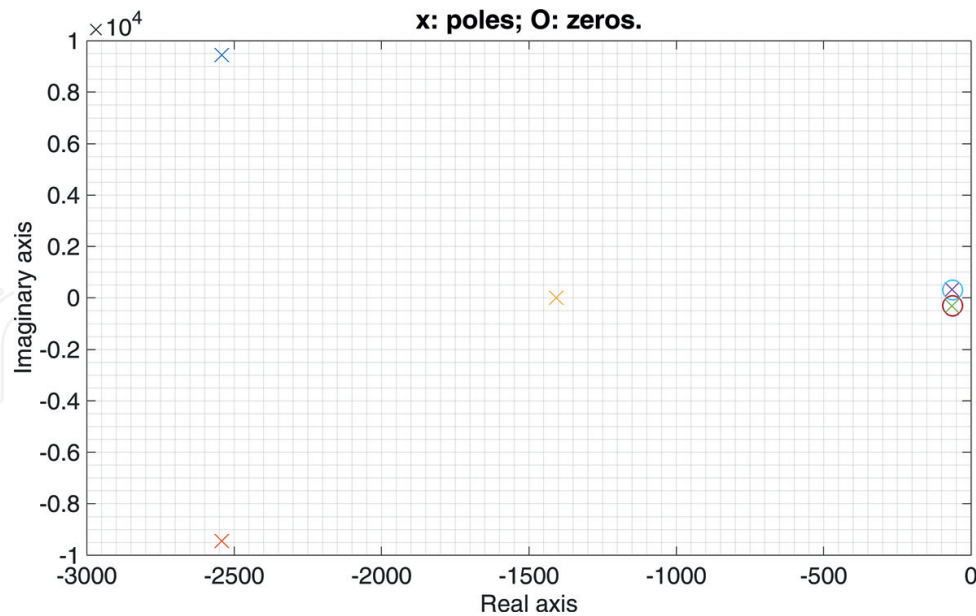
Figure 7. Designed zeros and poles of closed-loop transfer function using differential evolution optimization.
