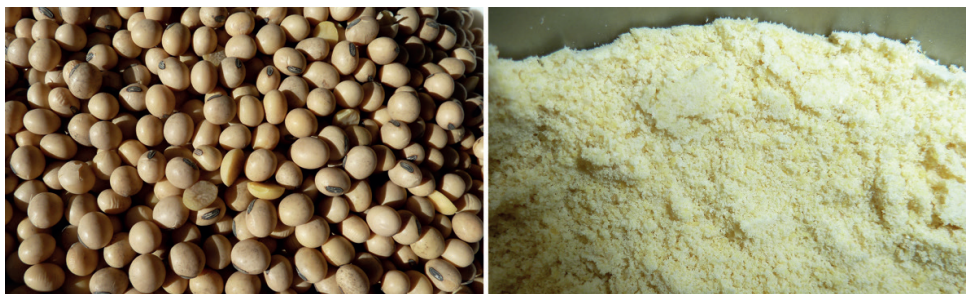
Figure 14. Homogenization of soy beans; left to right: original sample, sample ground to <500 μm.
