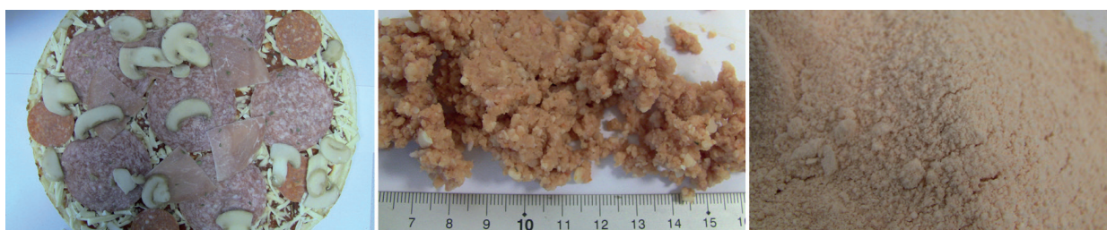
Figure 1. From left to right: a whole pizza; sample after grinding to coarse particles of <5 mm; fully homogenized sample with particle sizes of <0.5 mm.
