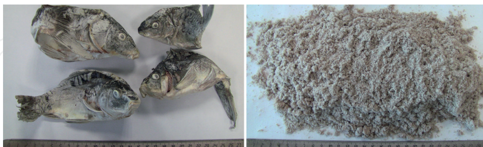
Figure 9. Homogenization of fish; from left to right: original sample, sample ground to <1 mm.
