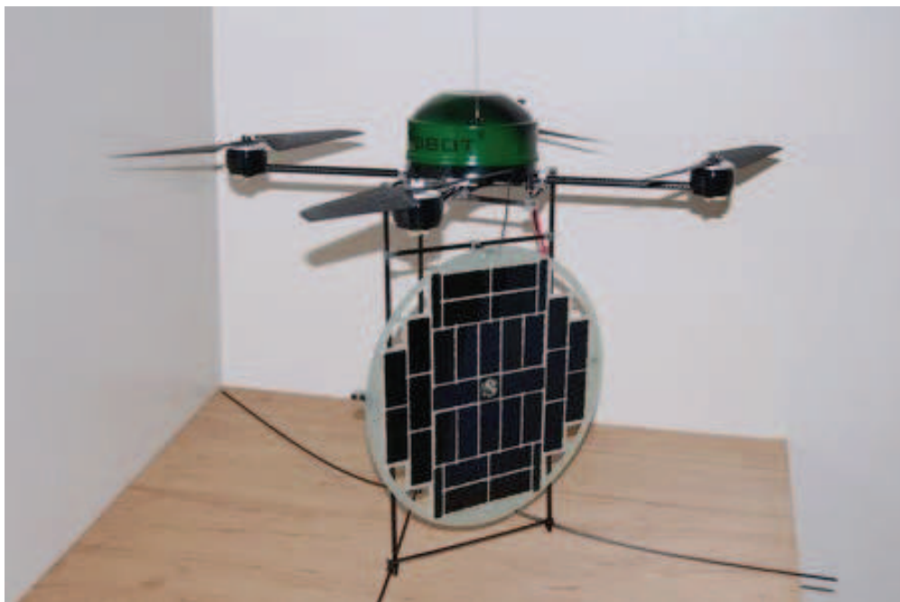
Fig. 8. Helicopter with a vertical solar panel underneath
