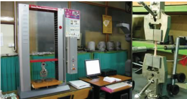
Figure 5. The determination of tensile mechanical resistance using the Zwick Roel extensometer.
