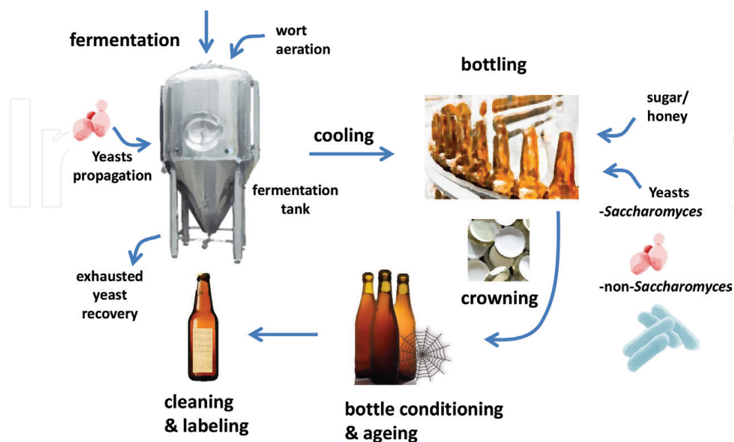
Figure 2. Brewing process: fermentation and bottle fermentation.
