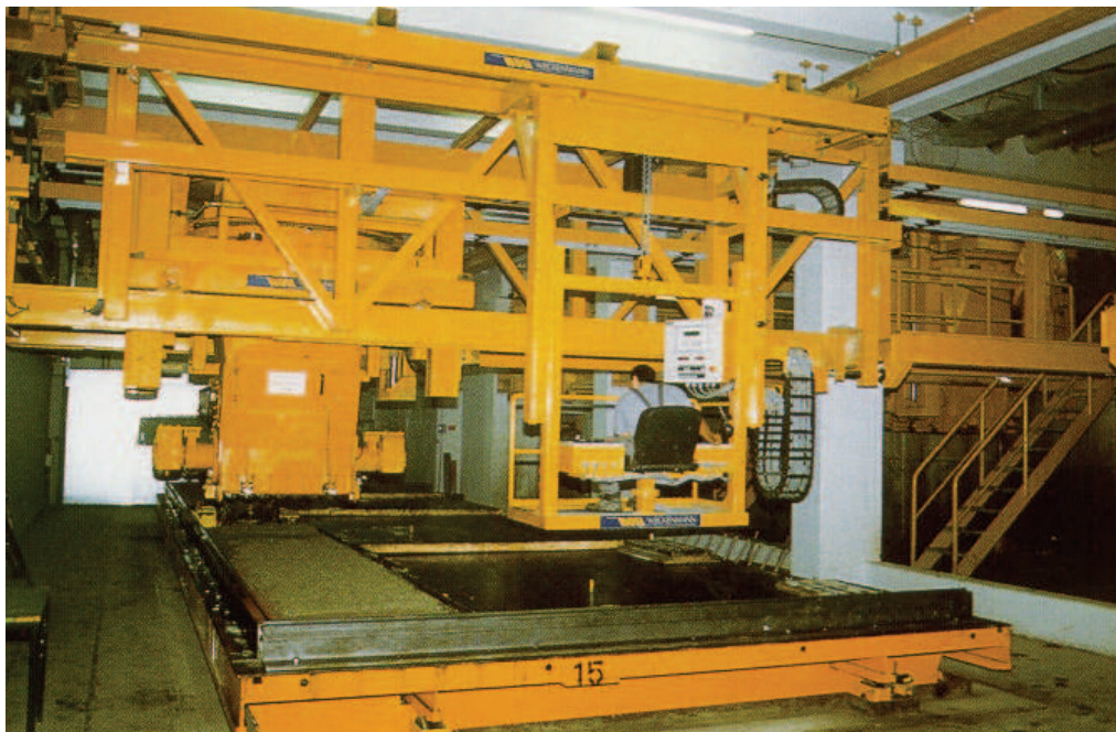
Fig. 4. Teleoperated concrete distribution
