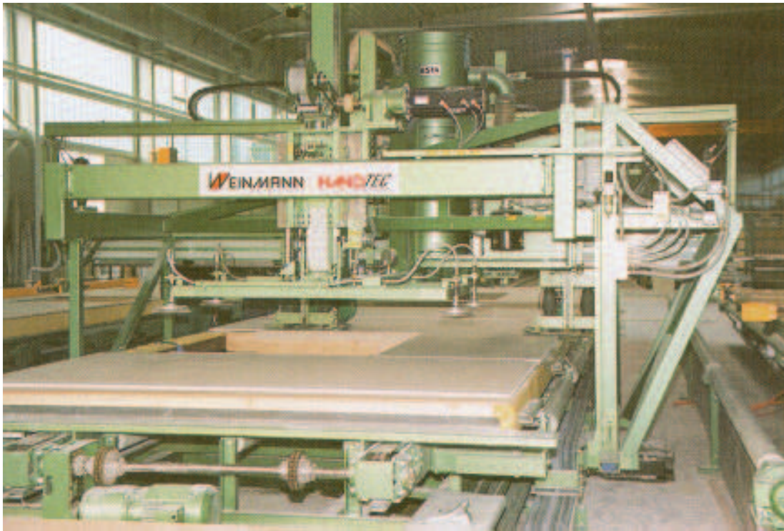
Fig. 5. Multifunctional robotic wooden wall production unit
