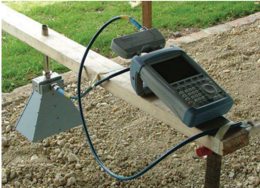
Figure 12. The UWB SFCW GPR system emulated using the hand-held VNA connected to the horn antenna via a 50-Ohm N-type coaxial cable.
