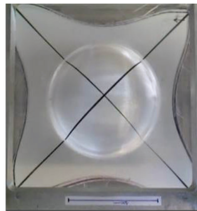
(b) The preform: [-45^\circ / +45^\circ]_4
