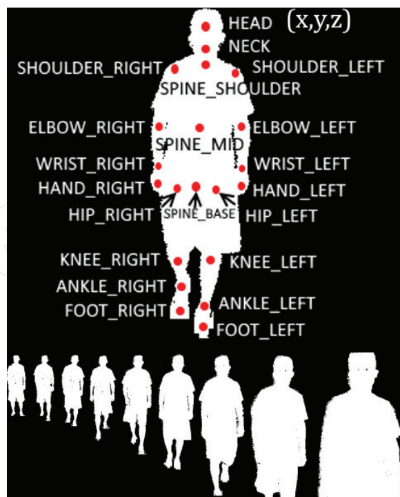
Figure 8. Two kinds of data in our database: 3D position of 21 joints in the upper area and the corresponding binarized silhouette images in the lower area.
