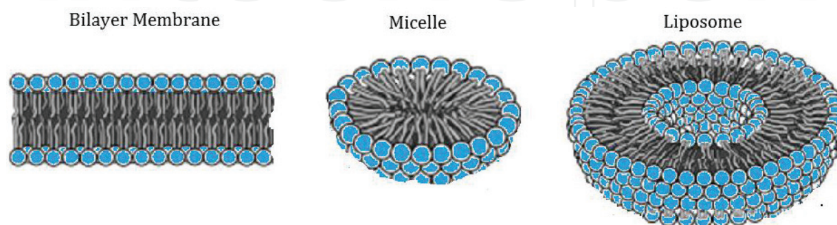
Figure 15. Various morphology of the polar and nonpolar arrangements in liposome and its formation.
