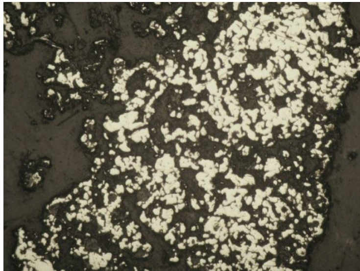
Figure 7. Microstructure of the periphery of the reduced BREX at a temperature of 1100°C: white, metal; gray, transformed mineral phases of the cement binder; reflected light, magnification \times 200 .
