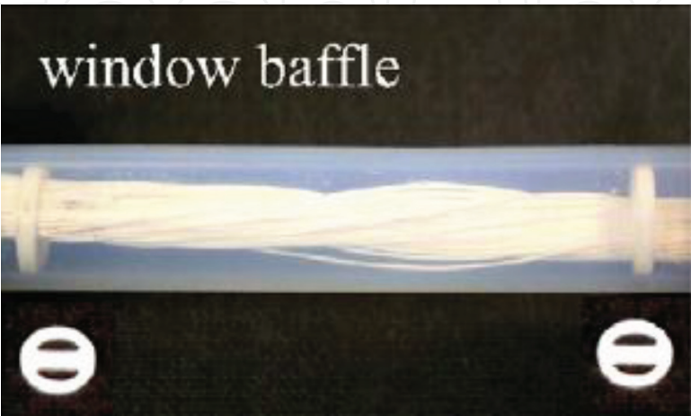
Figure 9. Hollow fiber module with window baffles [38].
