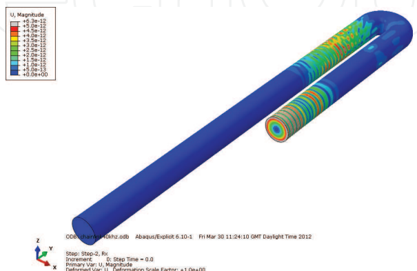
Figure 6. Displacement magnitude after propagation of a 10-cycle 40 kHz pulse around the bend.
