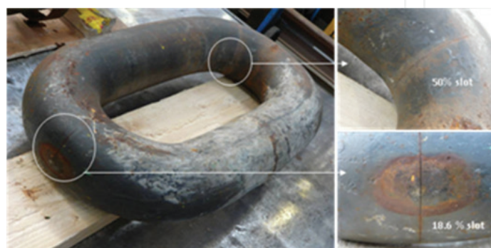
Figure 11. Aged chain link with slots.
