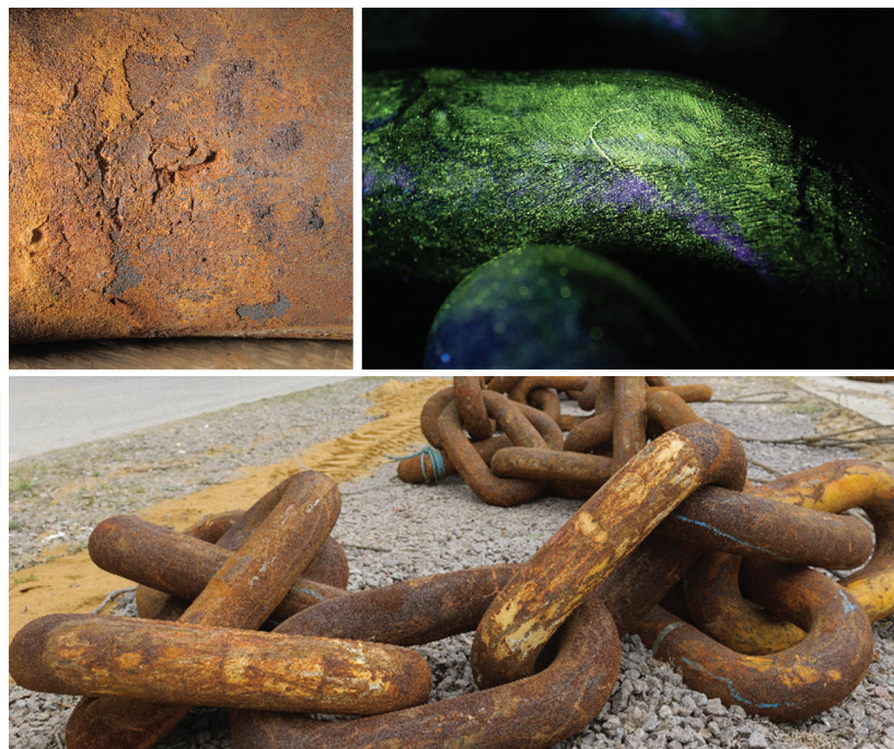
Figure 1. From left to right: Example of wear and corrosion on a chain link from the sea-bed touch down zone, in-water inspection showing a studded chain which has lost its stud in situ , illustration of marine growth on long-term deployed chain, affecting optical in-water inspection, friction-induced bending.
