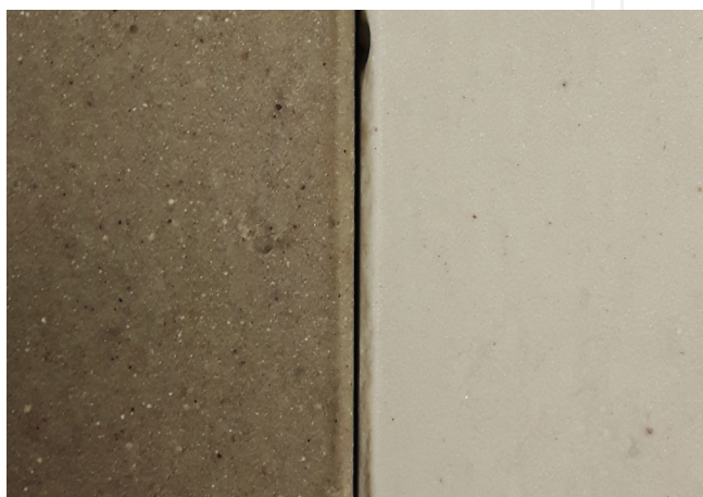
Figure 8. Color of sintered bodies with water absorption below 2%.
