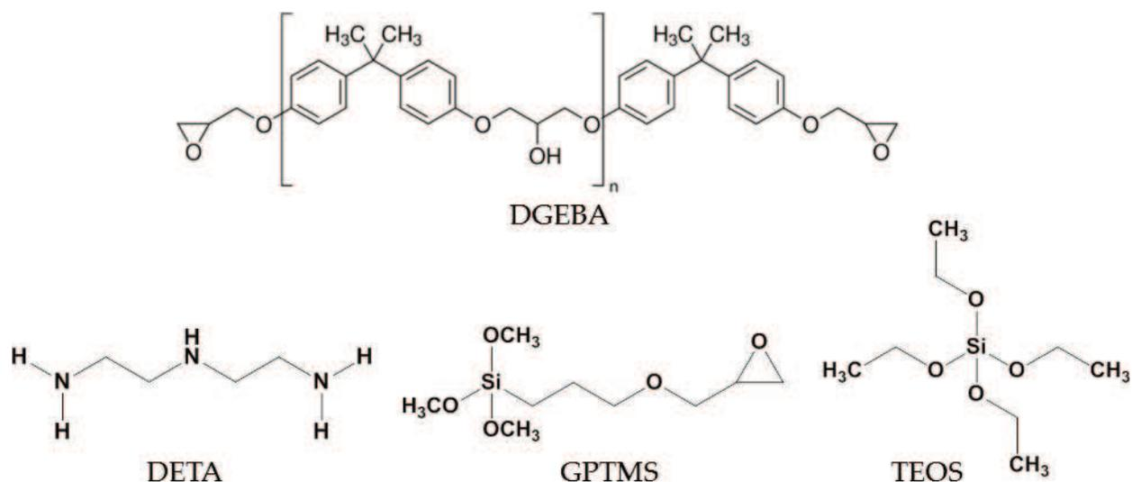
Figure 1. Molecular structures of the epoxy-silica hybrid precursors.
