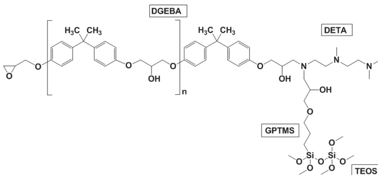
**Figure 8.** Molecular structure of the epoxy-silica hybrid.
