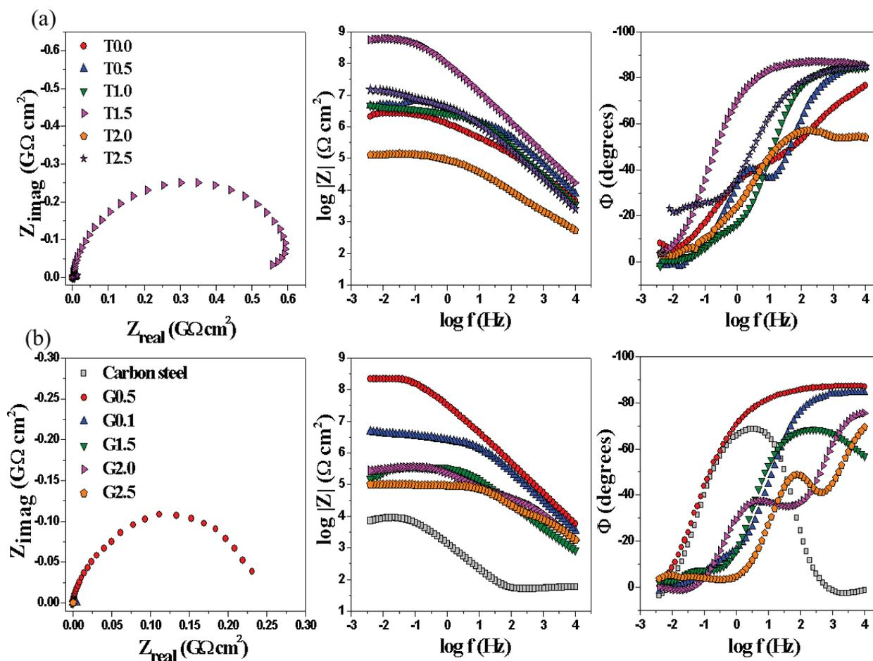
**Figure 12.** Nyquist and Bode plots of (a) series T and (b) series G of the epoxy-silica coatings deposited on carbon steel, compared to those of bare carbon steel, after 1 h of immersion in 3.5% NaCl solution.
