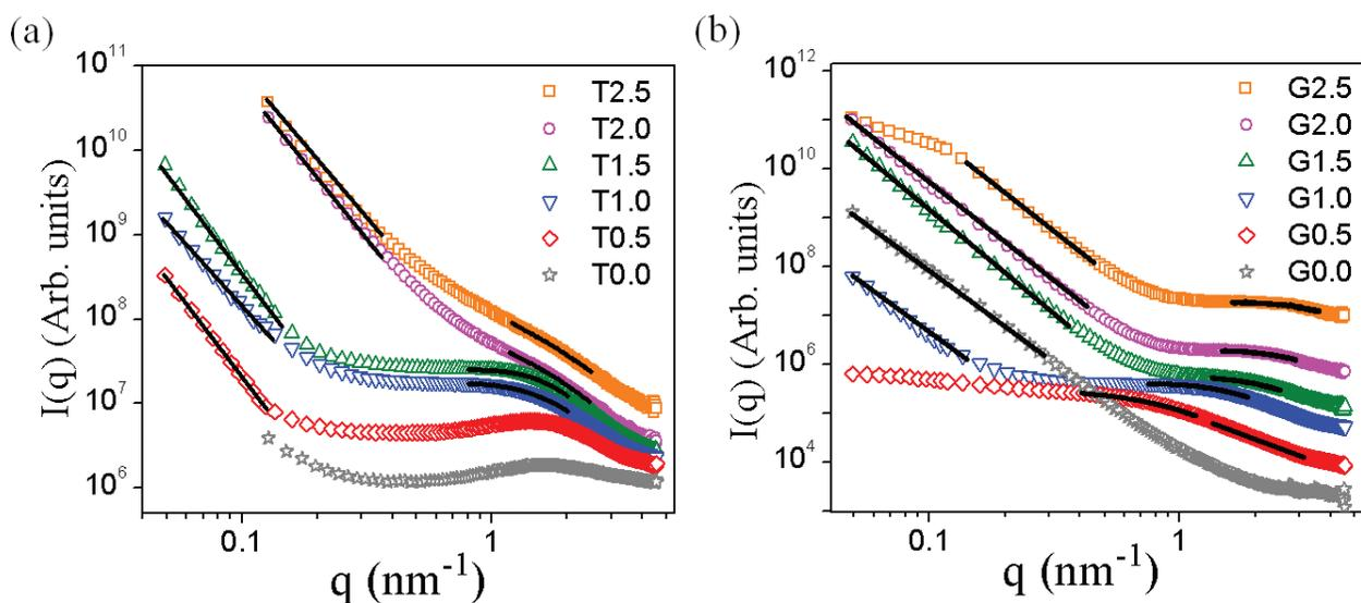
**Figure 11.** SAXS curves of T-series (a), and G-series (b), where the black lines represents the fits used to calculate the Porod coefficient ( $\alpha$ ) for  $q < 1$  (except for the G0.5 sample, which presents  $\alpha$  at  $q > 1$ ), and the radius of the gyration ( $R_g$ ) for  $q > 1$ . (The intensities were shifted to obtain a better visualization of the curves).
