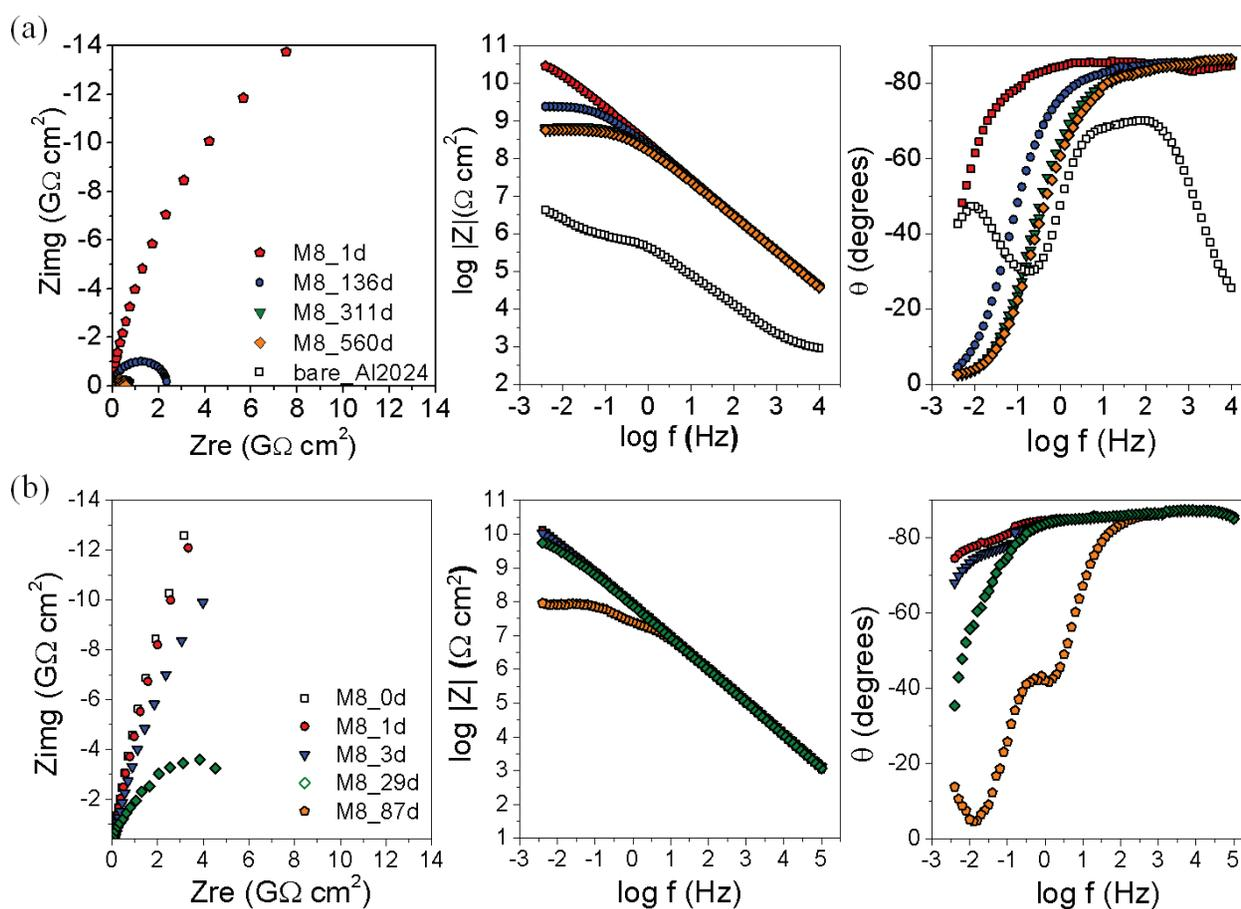
Figure 14. Time dependence of Nyquist and Bode plots of the M8\_T80BPO0.01 PMMA-silica coating deposited on Al2024 substrate in contact with a) in  $3.5\% \text{ NaCl}$  solution and b)  $0.05 \text{ mol L}^{-1} \text{ NaCl} + 0.05 \text{ mol L}^{-1} \text{ H}_2\text{SO}_4$  solution.
