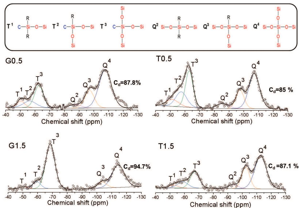
**Figure 10.**  $^{29}\text{Si}$ -NMR spectra obtained for epoxy-silica hybrids. Inset: schematic representation of the  $T^j$  and  $Q^j$  species, where 'R' indicates OH or  $\text{OCH}_3$  or  $\text{OCH}_2\text{CH}_3$  groups.
