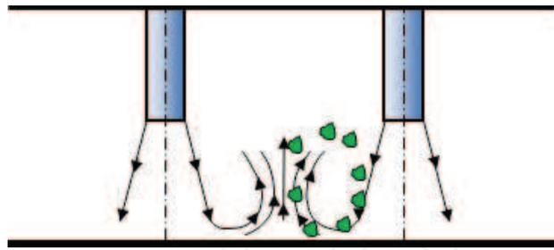
**Figure 4.** Motion of product in jet impingement fluidization.
