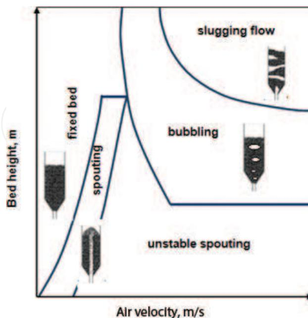
**Figure 2.** Ranges of the bed structures.
