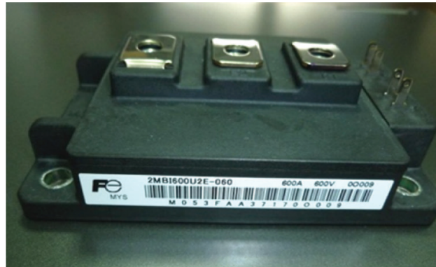
Figure 15. IGBT power transistors, T1/T2 type 2MBI 600 U2 E—060—FUJI [14].
