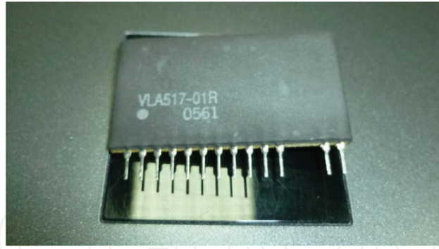
Figure 17. Hybrid integrated circuit, type VLA 517—01R—FUJI, driver [14].
