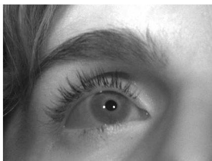
Figure 1. Image of the eye captured by the camera. The corneal reflections are the bright dots in the image
