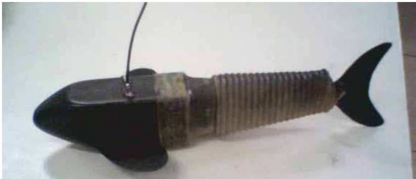
Fig. 2. Prototype of robot fish used in RWP
