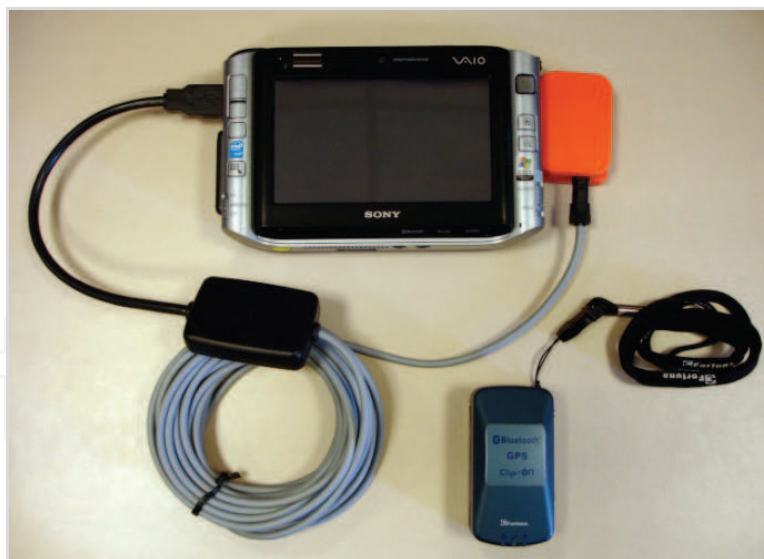
Figure 2. Ultra-mobile PC based hardware prototype
