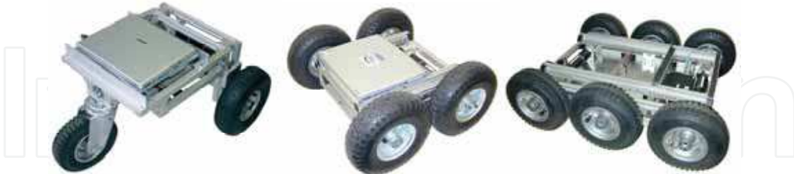
Fig.10. 3-wheeled, 4-wheeled and 6-wheeled variant of VolksBot RT
