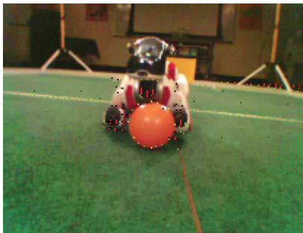
Fig. 7. The results of feature detection over a sample image. Ball edge features are displayed as yellow points, line edge features as light green points, obstacles as red points and field-green features as dark green points. Black points represent features that have been discarded due to checks applied after initial detection
