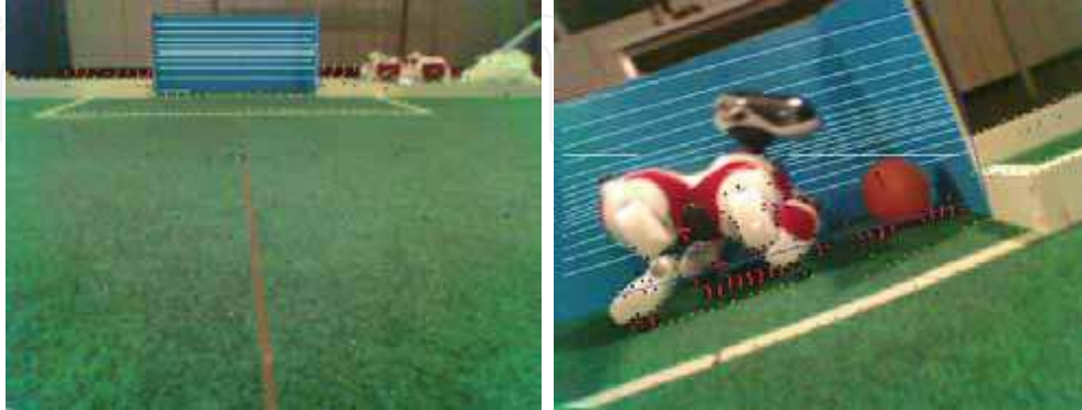
Fig. 9. (a) A recognised goal. (b) The goal is often occluded by a robot, but grouping of features leads to correct recognition, even if the goal is divided in half. The two possible gaps for shooting are indicated by horizontal white lines. The recognised goal is assumed to be aligned with the horizon, so no attempt is made to detect the goal outline
