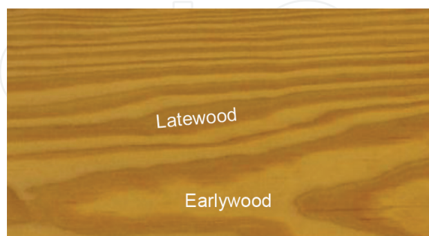
Figure 1. Image of flat-grained southern yellow pine wood showing distinctive wide earlywood and latewood sections.
