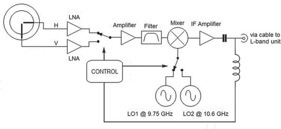
**Figure 3.** Universal low noise block (LNB) diagram.
