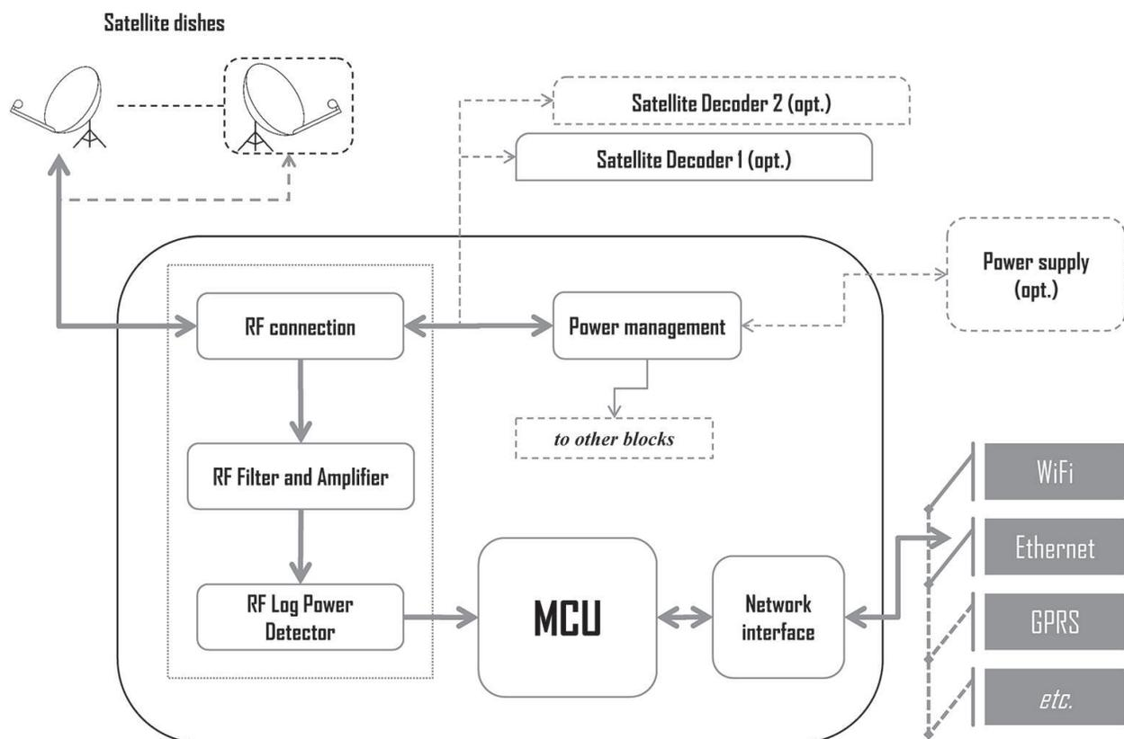
**Figure 2.** DVB-S power detector module.
