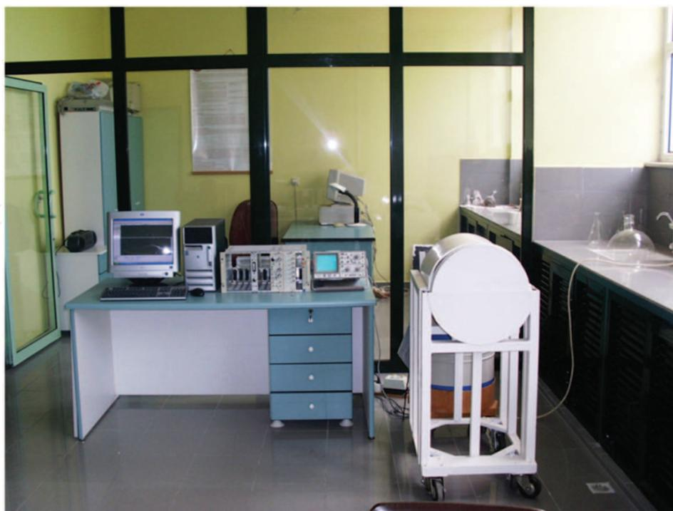
**Figure 1.** General appearance of the gamma-ray spectrometry system.
