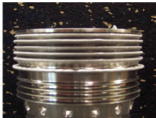
Figure 10. Laser repair technology of Inconel 718 compressor seal [17].
