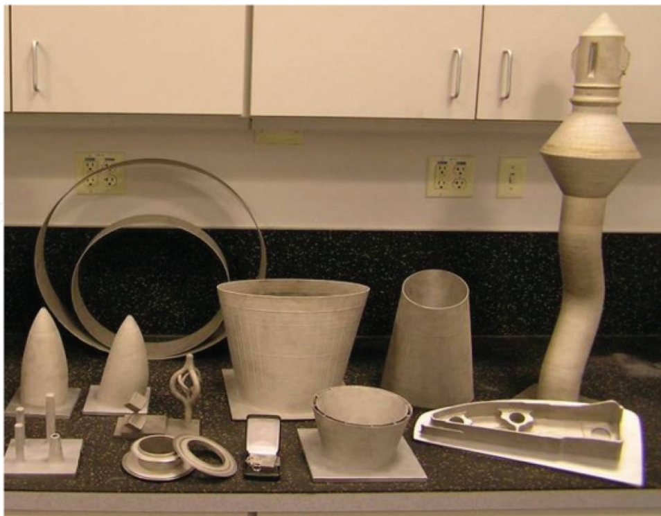
Figure 12. Examples of parts produced by free-form technology [18].
