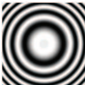
Figure 1. Interference pattern or interferogram showing circular fringes.
