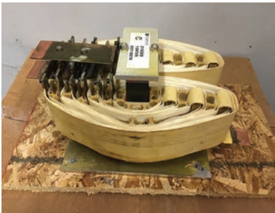
Figure 17. PWM 10 kW transformer dimensions 250 × 190 × 140 mm high.
