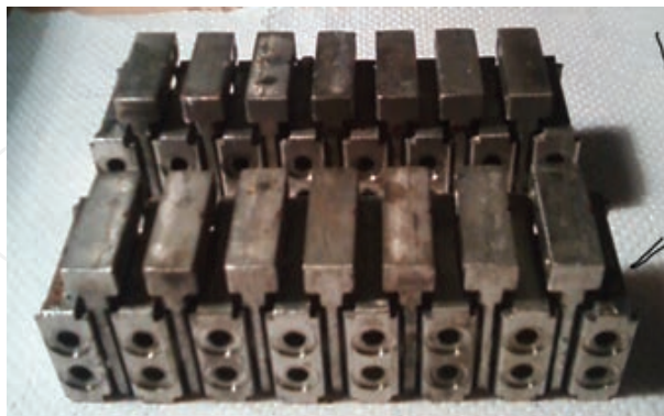
Figure 8. Thermoelectric column built by Nedelcu.
