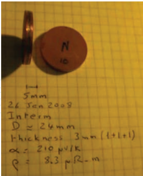
Figure 16. Bismuth telluride disc with copper caps.
