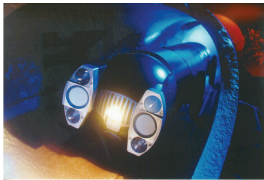
Fig. 2. The multi sensorial sewer inspection robot prototype, KARO
