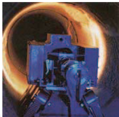
Fig. 1. The automated video inspection platform, PIRAT ( http://vision.cmit.csiro.au/project/pirat/ )
