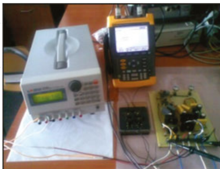
Figure 23. The microactuator with magnetic nanofluid during testing [68].
