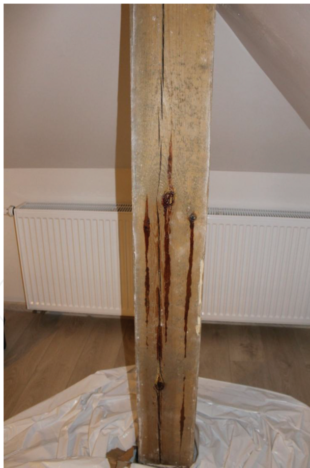
Figure 10. Resin melting in pine wood after exposure to microwaves radiated in practice by the 0.6 kW SAURUS device made in Italy (photo by CARSEKT).
