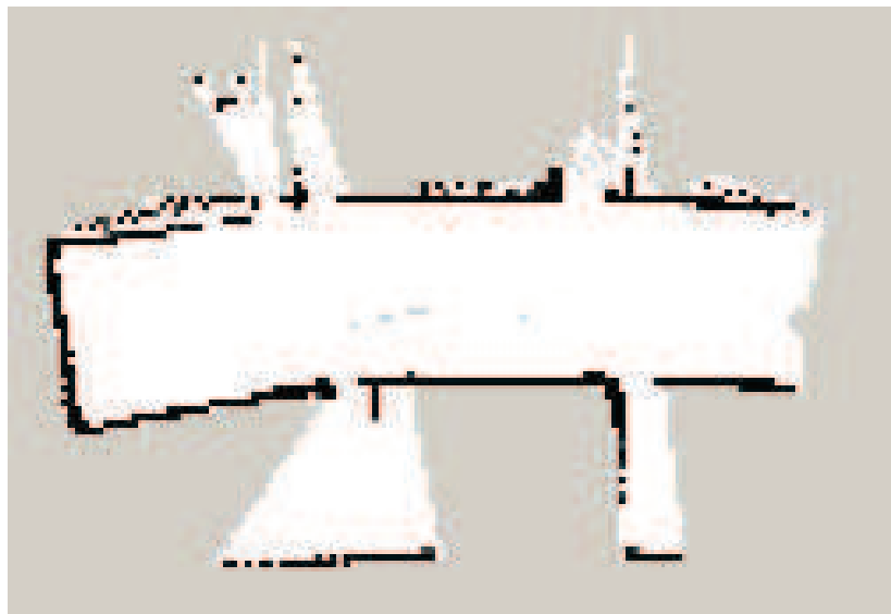
Fig. 1. Example of an occupancy grid map
