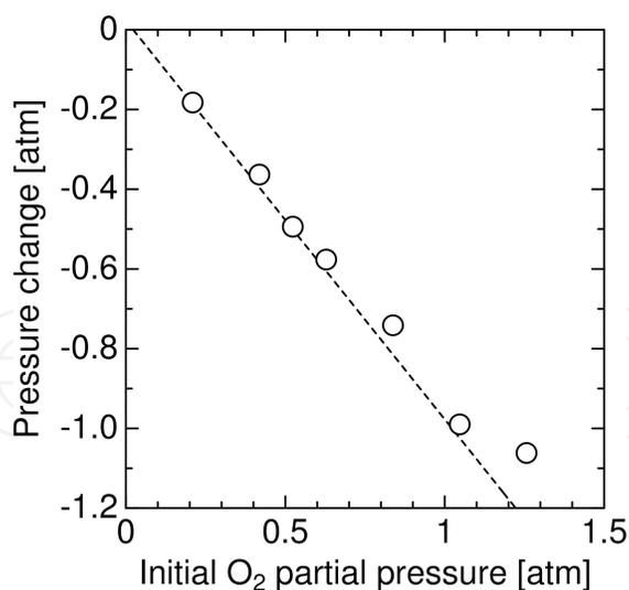
Figure 14. Change in the pressure after milling with the initial O<sub>2</sub> partial pressure.
