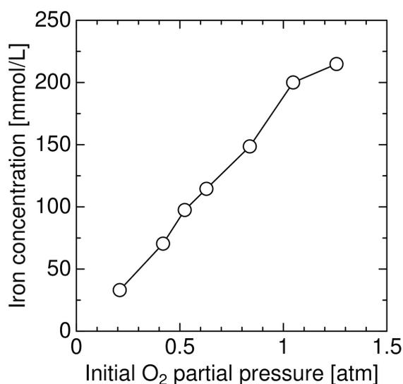
Figure 15. Change in the estimated iron concentration with the initial O<sub>2</sub> partial pressure.
