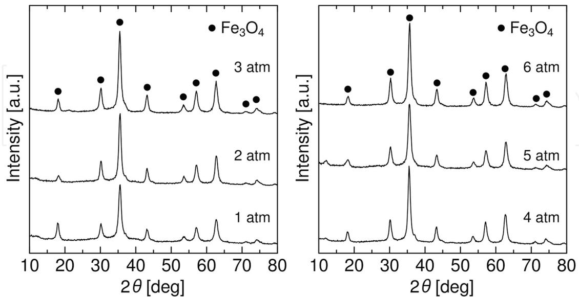
Figure 12. Effect of the initial total pressure on  $\text{Fe}_3\text{O}_4$  phase evolution.
