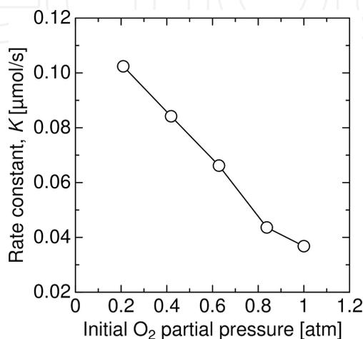
**Figure 18.** Change in the rate constant *K* with an initial O<sub>2</sub> partial pressure.
