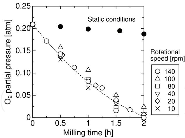
Figure 20. Effect of the rotational speed on the  $O_2$  partial pressure after milling.
