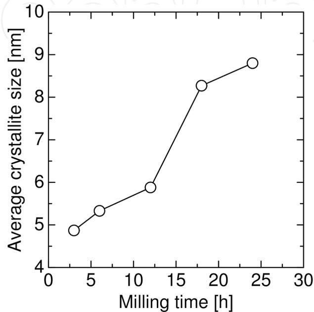
**Figure 2.** Change in the average crystallite size of Fe<sub>3</sub>O<sub>4</sub> with milling time.
