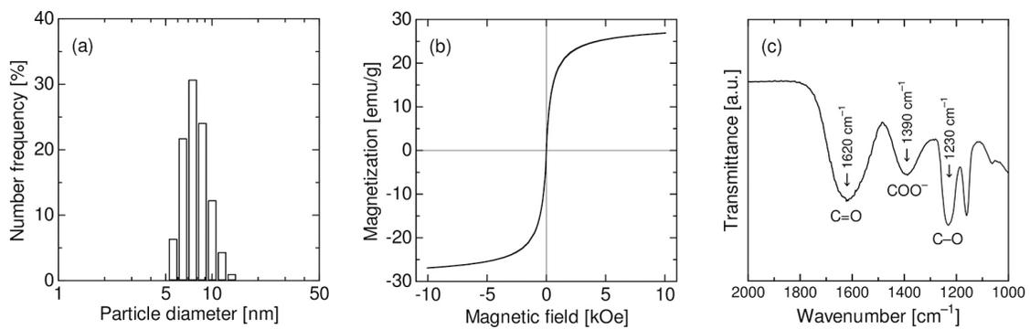
**Figure 5.** (a) Particle size distribution, (b) magnetization-magnetic field hysteresis cycle, and (c) FT-IR spectrum of the solid product.
