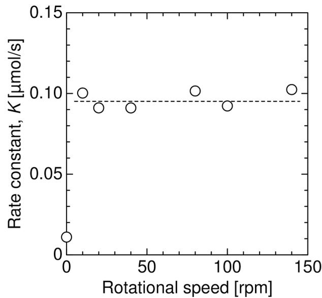
Figure 21. Effect of the vessel rotational speed on the rate constant  $K$ .
