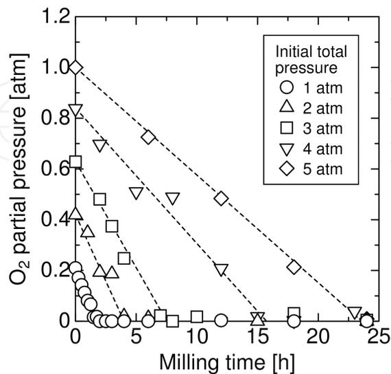
**Figure 17.** Change in the  $\text{O}_2$  partial pressure with a milling time of up to 24 h.
