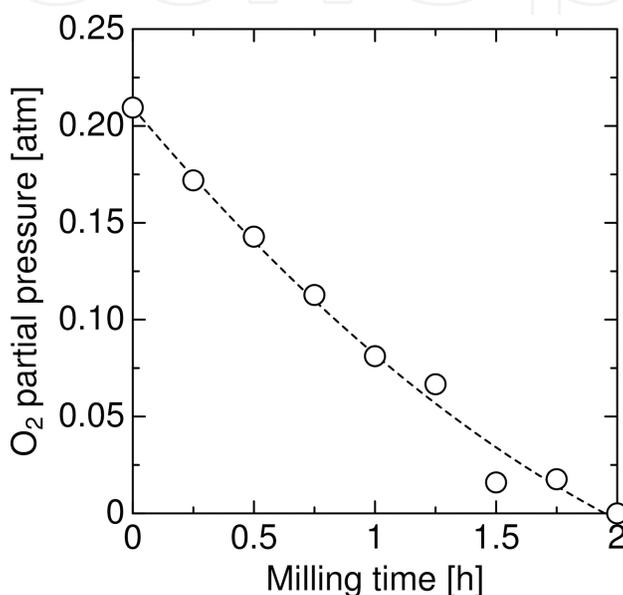
**Figure 16.** Changes in the O<sub>2</sub> partial pressure with milling time at an initial total pressure of 1 atm.
