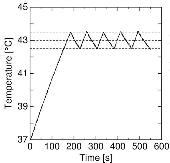
**Figure 6.** Temperature adjustment of the fluid in an on-off-controlled alternating magnetic field.
