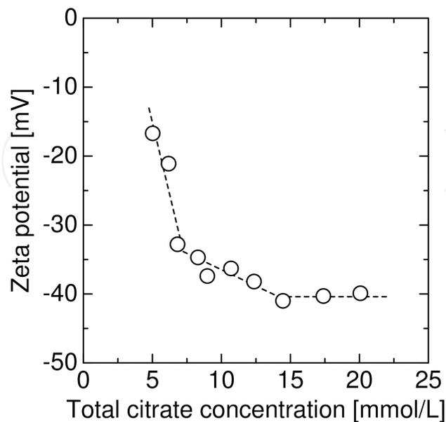
**Figure 3.** Effect of citrate concentration on the zeta potential of the fluid obtained with milling time of 18 h.
