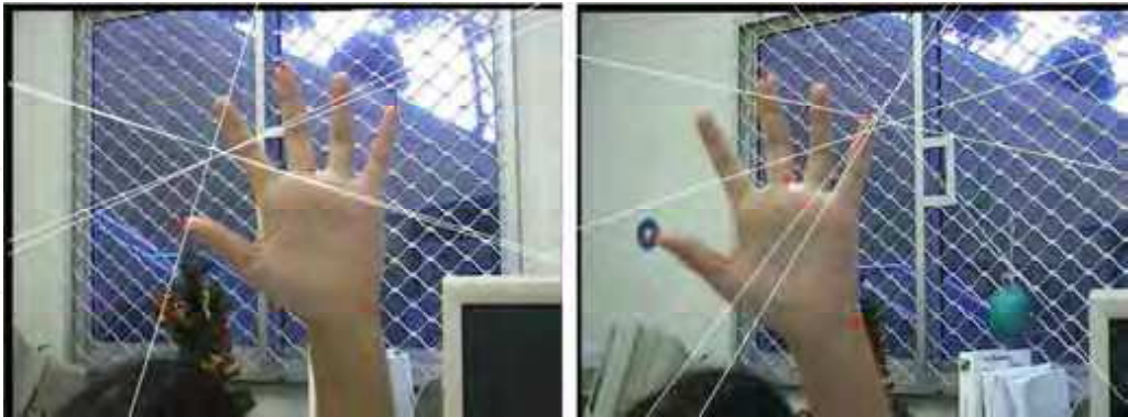
Figure 15. (a) Extracted matches using the method proposed by Zhang from uncalibrated hand images shown in Fig. 13, (b) Estimated epipolar geometry from these matches
