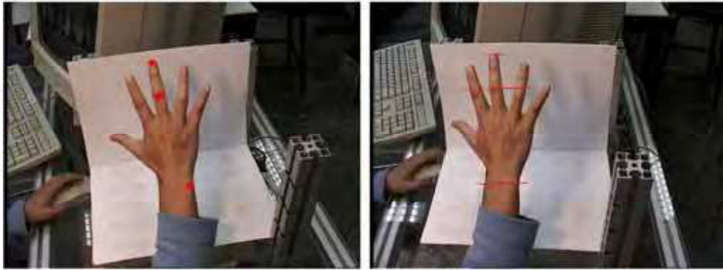
Figure 17. Find corresponding points in the right image which are marked by red points, for points in the left image which are marked by red crosses, using the color correlation and epipolar geometry
