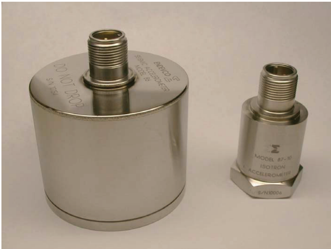
Figure 3. Photographs of the designed accelerometers [10, 13].
