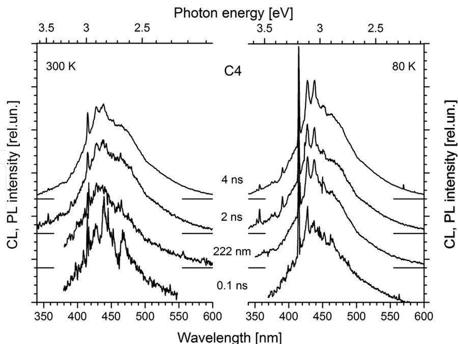
**Figure 7.** CL and PL integrated spectra of natural diamond IIa-type sample C4 at temperatures of 300 and 80 K. The CL excitation was provided by electron beams with durations of 0.1, 2, and 4 ns. The PL excitation was provided by KrCl-laser with pulse duration of 18 ns.
