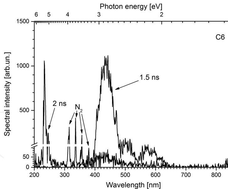
**Figure 9.** CL integrated spectra of polycrystalline CVD diamond sample C6 at room temperature. The CL excitation was provided by electron beams with pulse duration of 1.5 and 2 ns. The integrated spectrum obtained at 1.5 ns excitation was magnified in 30 times compared with the spectrum obtained at 2 ns excitation.
