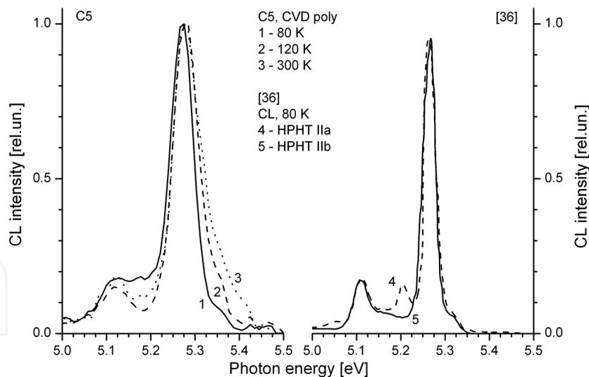
**Figure 12.** CL spectra of polycrystalline CVD diamond sample C5 at several temperatures from 80 up to 300 K at excitation by 2-ns electron beam (left part). CL spectra of two HPHT samples at 80 K from Ref. [36].
