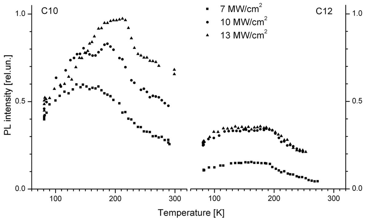
**Figure 18.** Temperature dependencies of FE recombination band intensities of two monocrystal diamond samples C10 and C12 at different excitation intensities at 222 nm. Squares-laser intensity 7 MW/cm<sup>2</sup>, circles-10 MW/cm<sup>2</sup>, triangles-13 MW/cm<sup>2</sup>.
