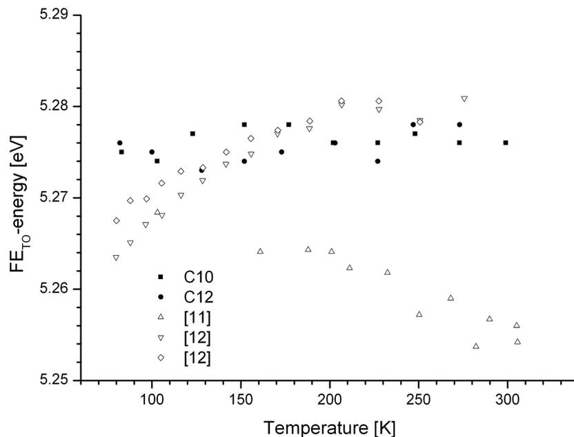
**Figure 4.** Positions of indirect optical transitions depending on diamond sample temperature. Excitation was provided at 222 nm with peak intensity 1 MW/cm<sup>2</sup>. Black squares-sample C10, black circles-sample C12, open triangles-data from Ref. [11], open turned triangles and open rhombs-data from Ref. [12].
