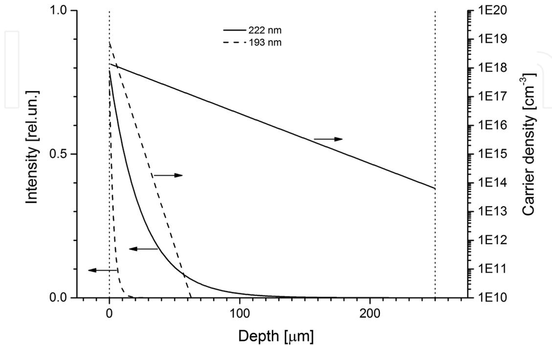
**Figure 2.** Laser intensity and charge carrier density in the diamond sample C5 versus the depth of sample for laser excitation on 222 nm (solid curves) and 193 nm (dashed curves).
