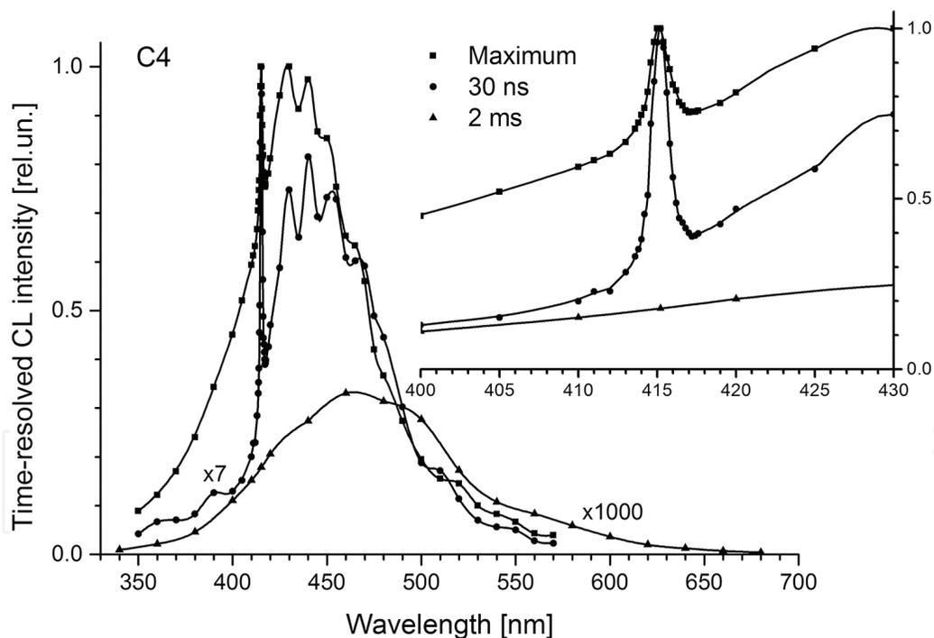
**Figure 10.** CL spectra of natural diamond sample C4 at room temperature obtained at 10 ns excitation. CL spectra were reconstructed at different wavelength (the method see in Ref. [29]) from the maximum of CL emission signals (squares), after 30 ns from the excitation starting (circles) and after 2 ms from the excitation starting (triangles). On the inset, there are CL spectra in the magnified spectral scale.
