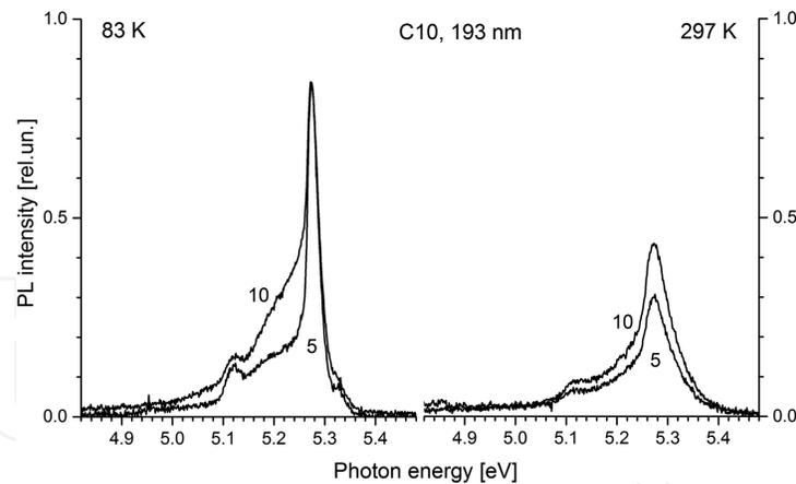
**Figure 16.** PL spectra of monocrystal CVD diamond sample C10 under the excitation at 193 nm at temperatures of 83 and 297 K. The PL spectra marked by peak intensities [5 and 10 MW/cm<sup>2</sup>] of laser radiation on the sample surface.
