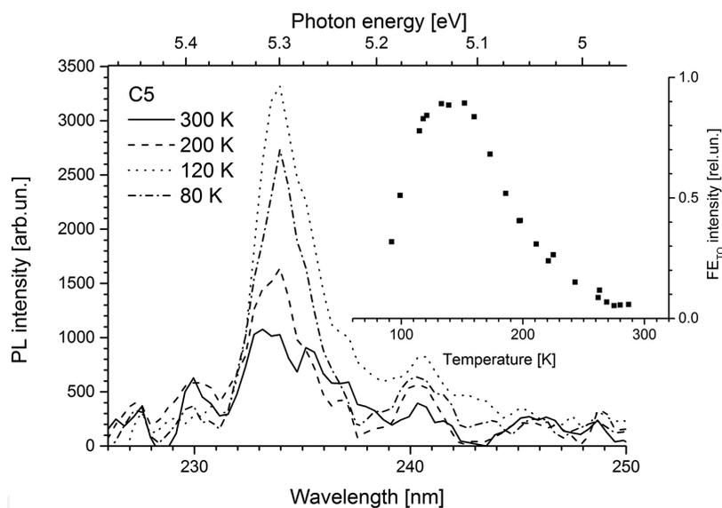
**Figure 6.** PL integrated spectra of polycrystalline CVD diamond sample C5 at different temperatures. The PL excitation was provided by KrCl-laser (222 nm) with pulse duration of 18 ns. On the inset there is the temperature dependence of FE band intensity of diamond sample C5.
