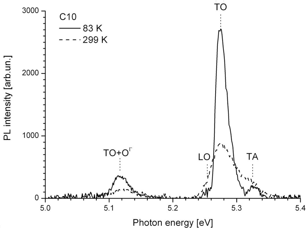
**Figure 3.** PL integrated spectra of diamond monocrystal C10 under excitation at 222 nm at temperatures of 83 K (solid curve) and 299 K (dashed curve). The spectrum contains the phonon components: TA (87 meV) at 5.325 eV, TO (141 meV) at 5.275 eV, LO (156 meV) at 5.254 eV and TO+O<sup>Γ</sup> (141 + 159 meV) at 5.117 eV.
