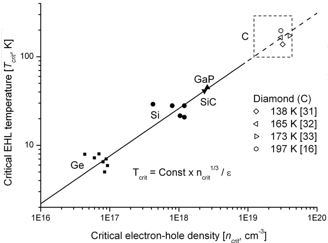
**Figure 20.** Critical EHL temperatures versus critical EHL densities in the several semiconductors. Black squares-germanium (Ge), black circles-silicon (Si), black down triangle-silicon carbide (SiC), black up triangle-gallium phosphite (GaP), white shapes-diamond (C). Data for Ge, Si, SiC and GaP referred to [30, 32], data for C (diamond)—[16, 31–33].
