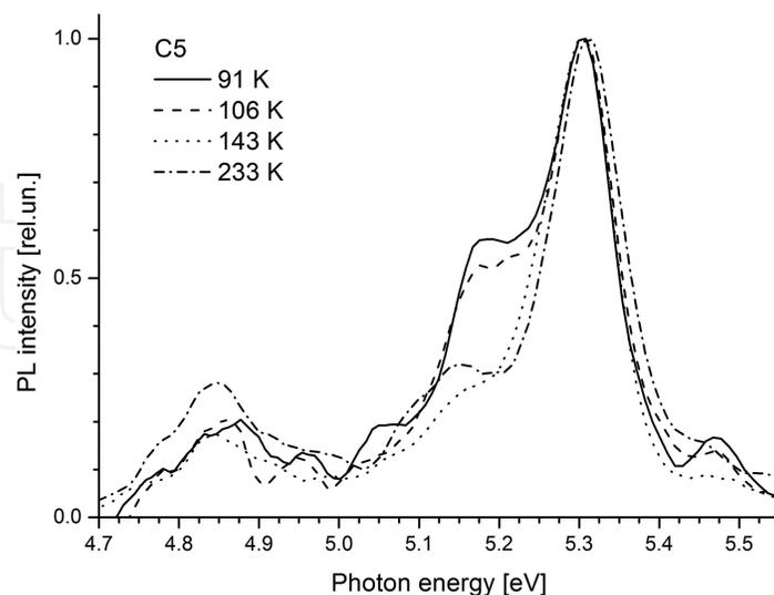
**Figure 13.** PL spectra of polycrystalline CVD diamond sample C5 at several temperatures from 80 K up to 300 K at excitation by 18-ns laser pulses at 222 nm with peak intensity 3 MW/cm<sup>2</sup>. The TO-component of FE band at 5.27 eV dominated in PL spectra. The TO-component of EHL band in the spectral range 5.1–5.2 eV was appeared on the long-wavelength edge of FE band.
