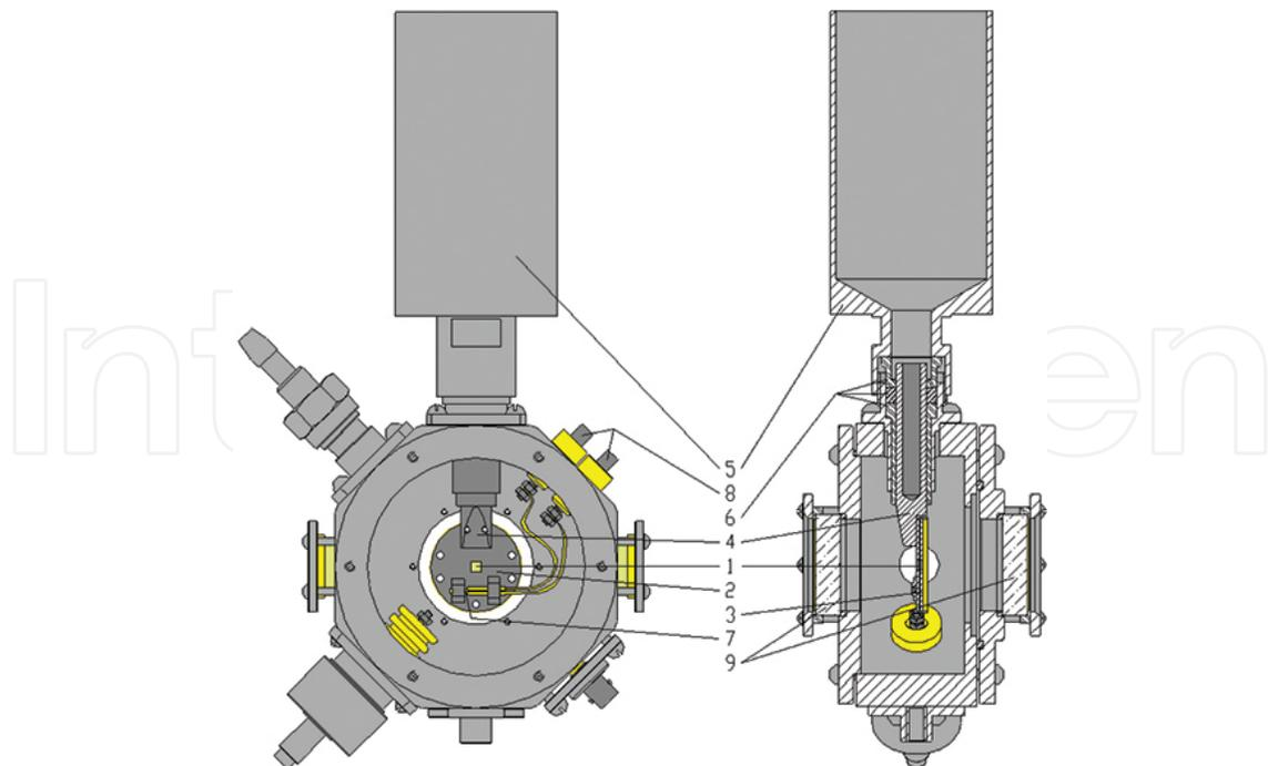
**Figure 1.** Vacuum chamber. 1-diamond sample; 2, 3-copper round plates; 4-hollow copper heat sink; 5-metal cup with liquid nitrogen; 6-seals; 7-platinum thermistor; 8-vacuum-tight electrical bushings; 9-fused silica windows.
