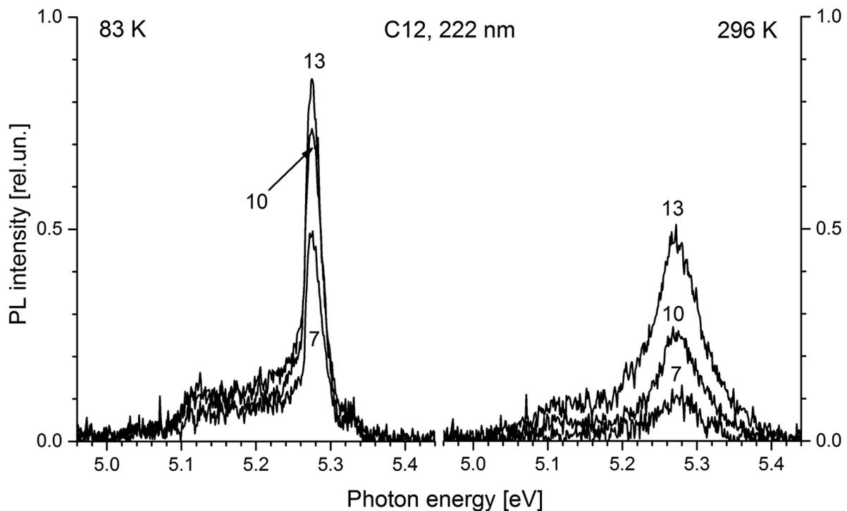
**Figure 17.** PL spectra of monocrystal HPHT diamond sample C12 under the excitation at 222 nm at temperatures of 83 K and 296 K. The PL spectra peaks are marked by peak intensities [7, 10 and 13 MW/cm<sup>2</sup>] of laser radiation on the sample surface.
