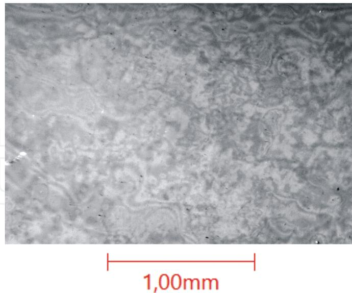
**Figure 14.** The microphotograph of surface of polycrystalline CVD diamond sample C5 with magnification  $\times 4$ . The crystallite sizes take values from 50 up to 400  $\mu\text{m}$ .
