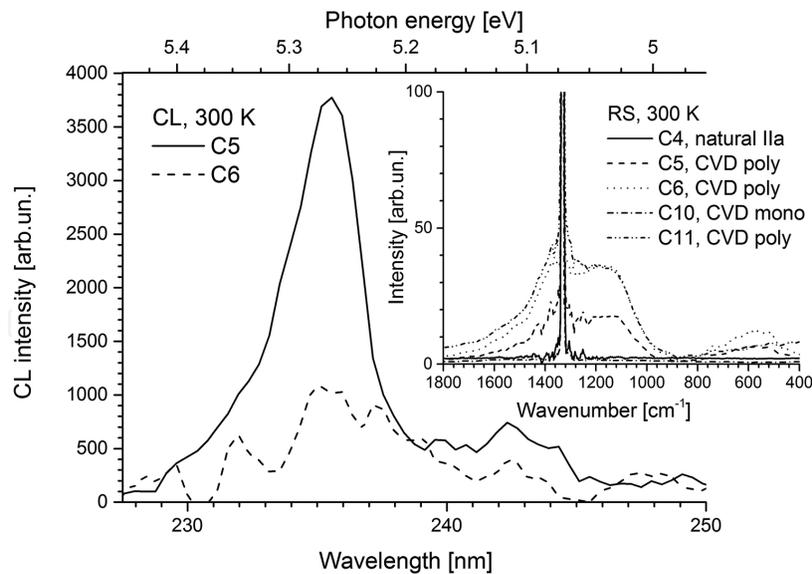
**Figure 5.** CL integrated spectra of polycrystalline CVD diamond samples C5 and C6 at room temperature. The CL excitation was provided by high-current electron beam (220 keV) with pulse duration of 2 ns. On the inset Raman spectra of several diamond samples at room temperature are shown.
