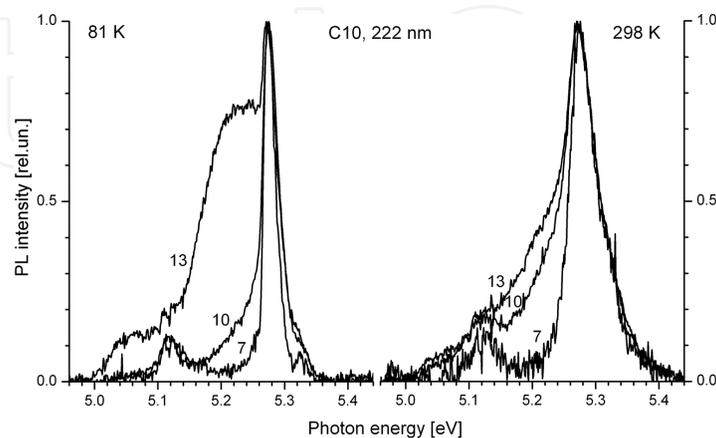
**Figure 15.** PL spectra of monocrystal CVD diamond sample C10 under the excitation at 222 nm at temperatures of 81 and 298 K. The PL spectra marked by peak intensities [7, 10, and 13  $\text{MW/cm}^2$ ] of laser radiation on the sample surface.
