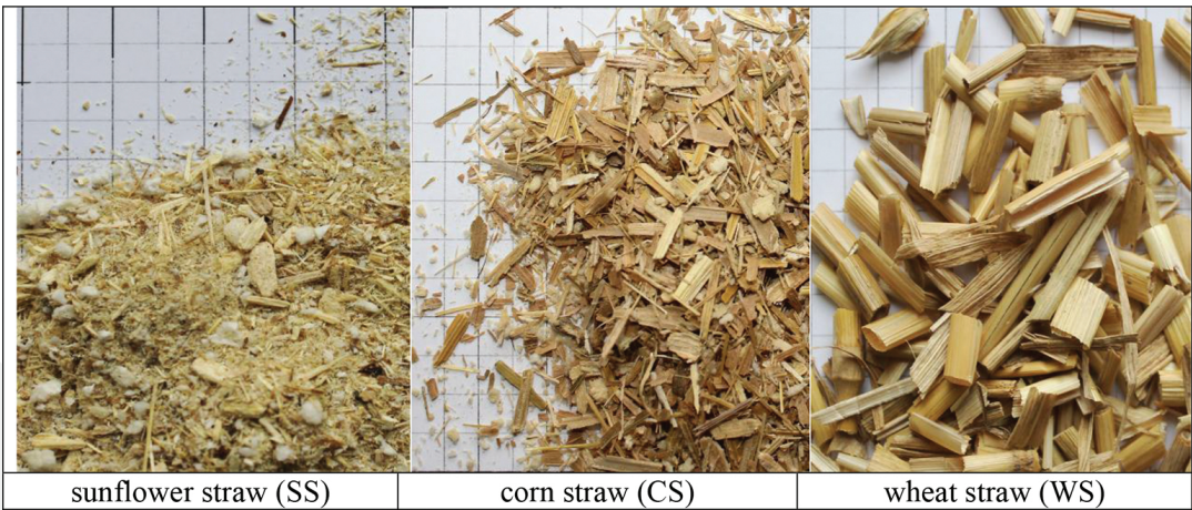
Figure 2. Photographs of the straw reinforcement.
