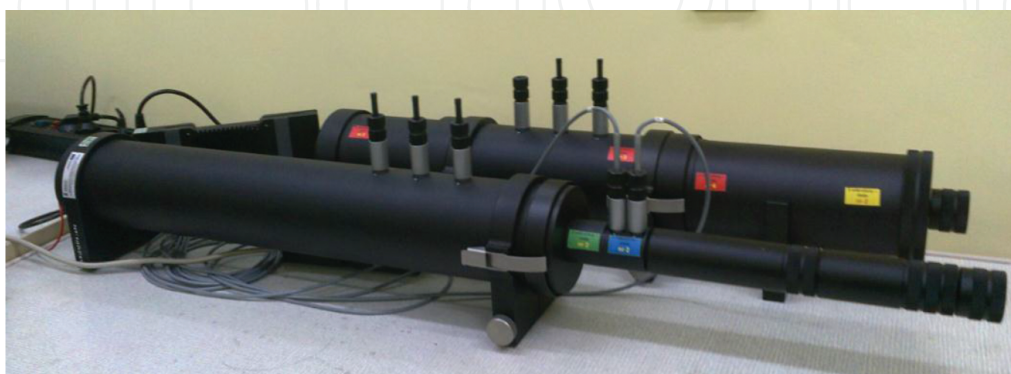
Figure 6. The Kundt device for acoustic measurements.
