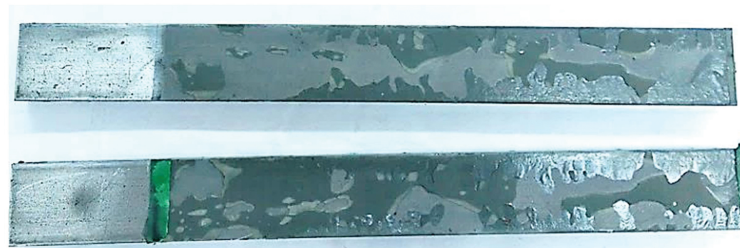
Figure 9. Failure surfaces for the DCB specimen.
