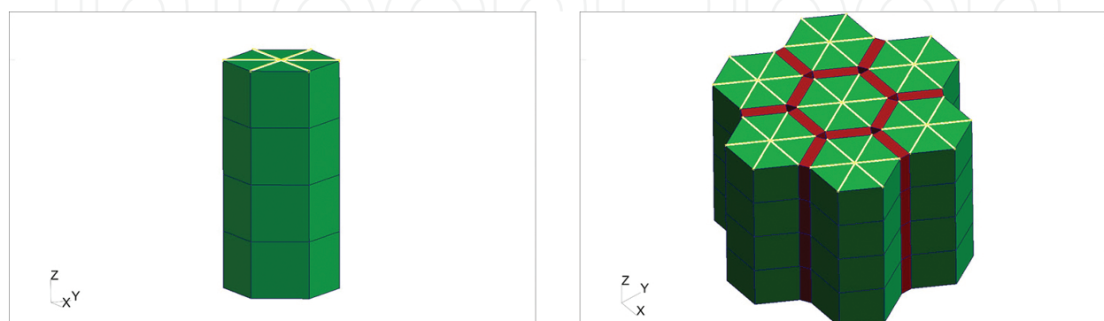
Figure 6. Single-cell model (left) and adherens junction model (right): diagonals of the top hexagon imitate actin fibres, red areas between cells imitate junction bonds.
