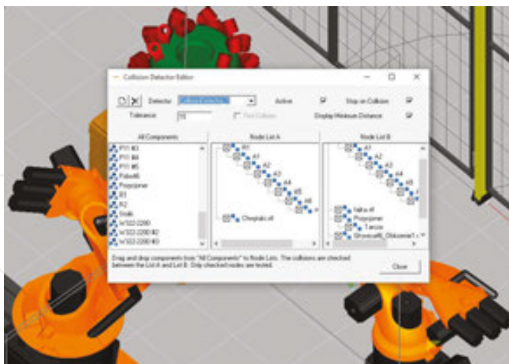
Figure 11. Collision detection module in KUKA.SimPro environment.
