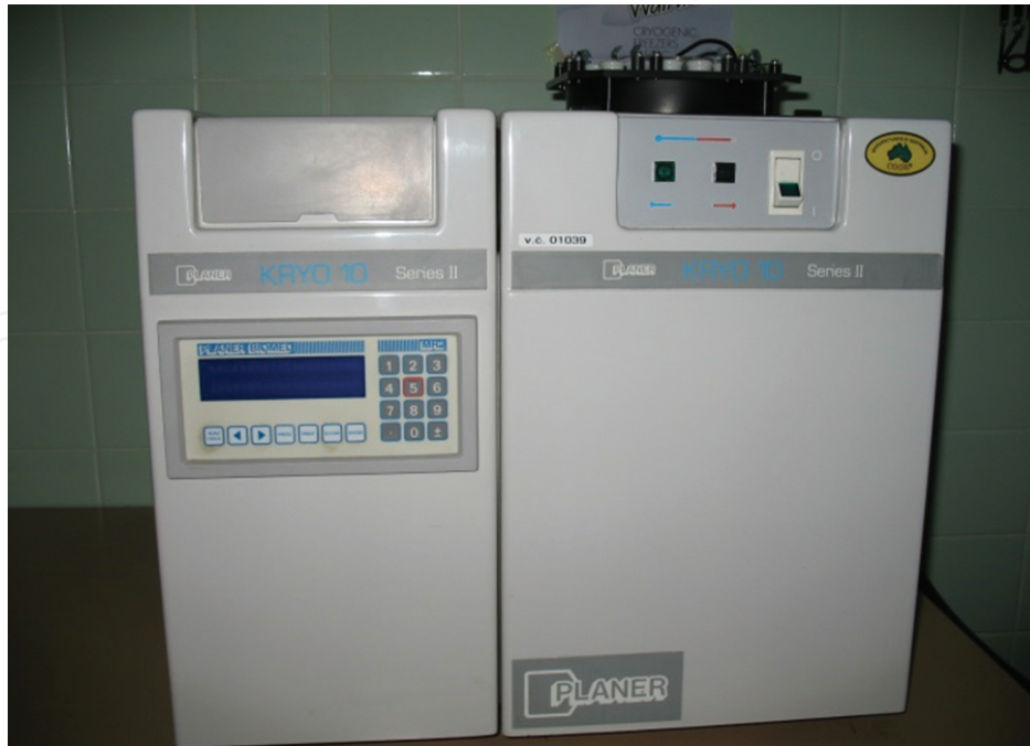
Figure 2. Programmable cryo freezer Planer Kryo F10.
