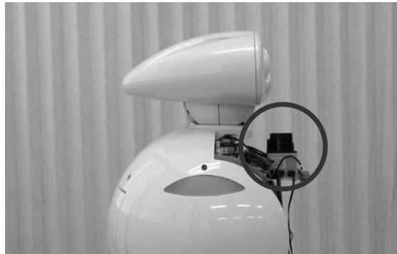
Fig. 11. LRF on ApriAttenda™ (side view)
