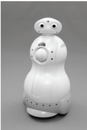
Fig. 1. Person Following Robot ApriAttenda™ (without LRF)
