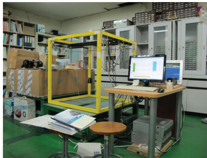
Figure 5. Overhead crane system used for the experiments.
