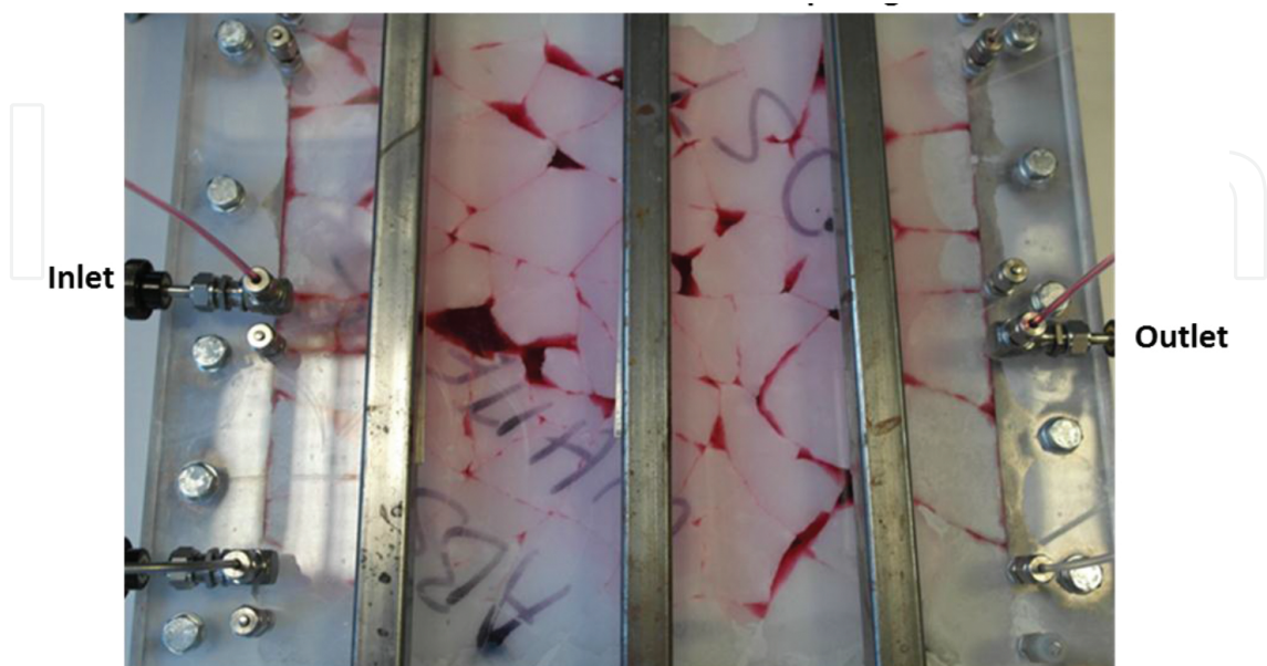
Figure 6. A square marble tile was fractured and reassembled within an aluminium frame sandwiched between two Plexiglas plates. The fracture network consisted mainly of narrow fractures with 12 large fractures. The vugular open fractures were larger bodies of open space varying between 0.4 and 2.2 cm aperture. These cavities were used to observe the advancing foam front during co-injection. In this figure, the marble tile model is filled with red-dyed brine to emphasize the fracture network.
