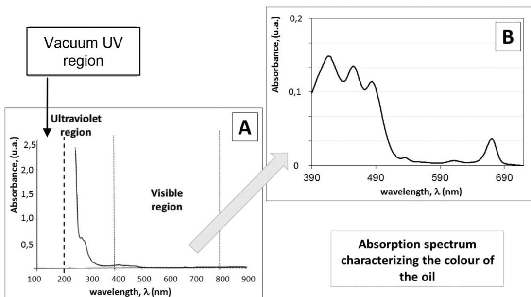
**Figure 3.** (A) Full experimental spectrum in the UV-vis region of an extra-virgin olive oil, showing the two separated regions: UV and Vis one. (B) Enlargement of the spectrum in the sole Vis region showing the typical shape of the Vis absorption spectrum of extra-virgin olive oils, due to the pigments content and responsible of the colour.
