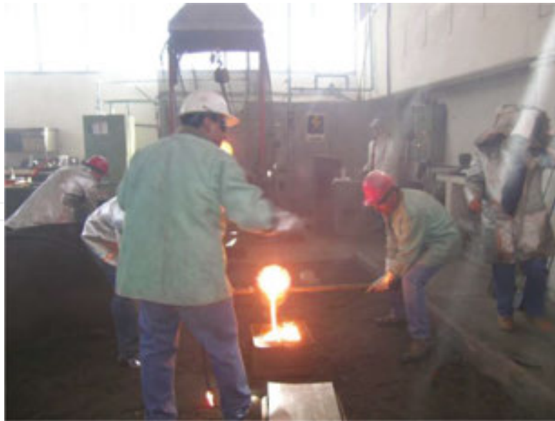
Figure 11. Pouring the liquid iron into sand moulds.
