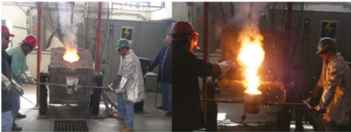
Figure 9. Pouring the liquid iron into the preheated ladle in the ductile iron making.
