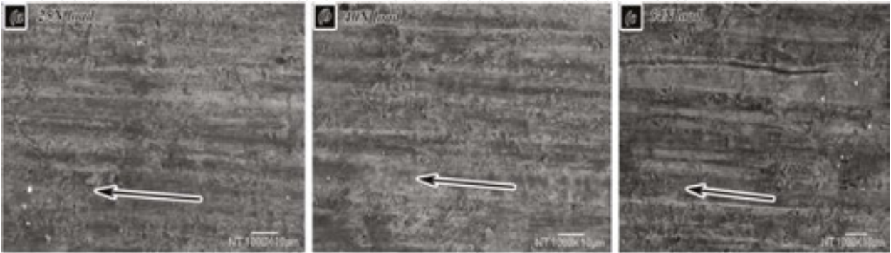
Figure 21. SEM micrographs showing the worn surface of an as-cast white iron after an abrasive wear test at three different loads, and evidencing the increase in roughness as load increases. The arrows indicate the wear direction [103].
