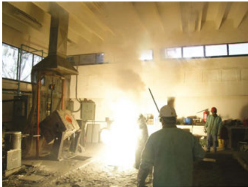
Figure 10. Nodulising ductile iron with magnesium, note the intensity of the reaction when magnesium is added into the liquid metal.
