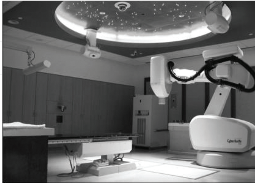
Figure 6. The Cyberknife VSI system installed in a clinical setting. Note the two X-ray tubes mounted on the ceiling and the X-ray detectors that are placed beneath the floor of the treatment vault for stereotactic imaging and on-line tracking.
