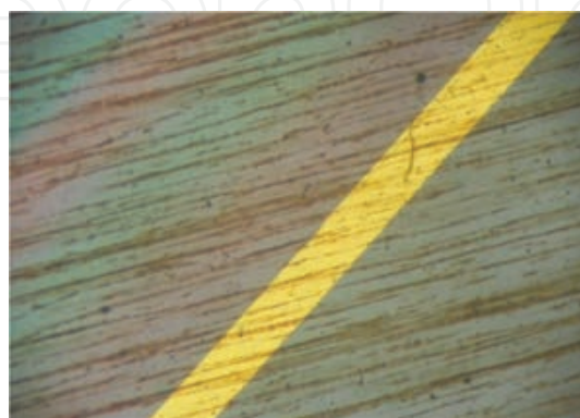
Figure 12. Microscopy image of 0.016 wt.% SWNT- \text{COOH} , 0.016 wt.% \text{Fe}_2\text{O}_3 in DI water. At 8 min, the internal reference is 30 \mu\text{m} . From Ref. [70].
